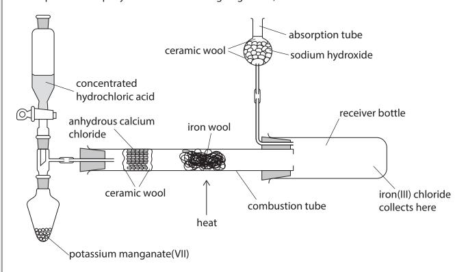
(a) Chlorine is generated by the vigorous redox reaction between concentrated hydrochloric acid and potassium manganate(VII). The chlorine moves through the apparatus as it is generated.
