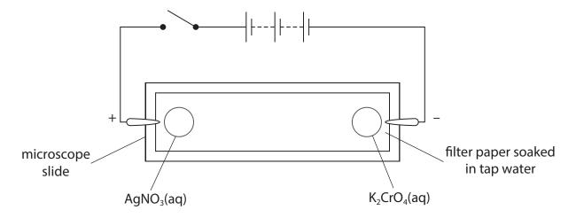
Several drops of aqueous silver nitrate and aqueous potassium chromate(VI), both of concentration 1.0 mol dm<sup>-3</sup>, were placed on the filter paper and the switch closed. After a short while, a red precipitate formed in the centre of the filter paper.
